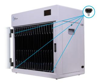
To configure racks differently, remove thumb screws from the left/right sides and pull the shelf out. Insert new shelf and replace thumb screws.
