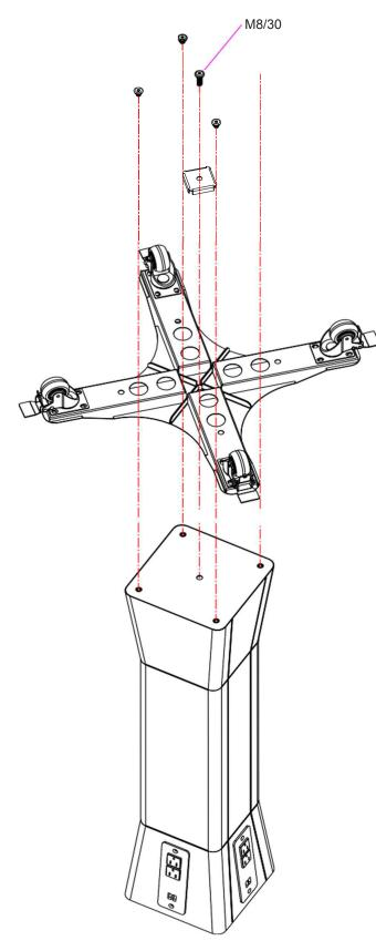
Place the unit on its top. Please place the top on a soft surface or padding to avoid damage to the top of the unit, and battery switch and display screen on BA versions
