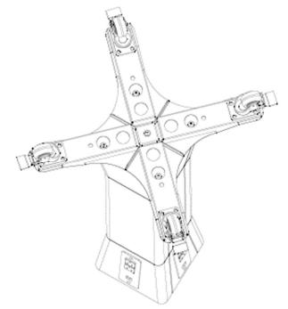
Note: AC-COLLABR-8<sup>™</sup> has low center of gravity which provides stability when moving and avoids tipping.
