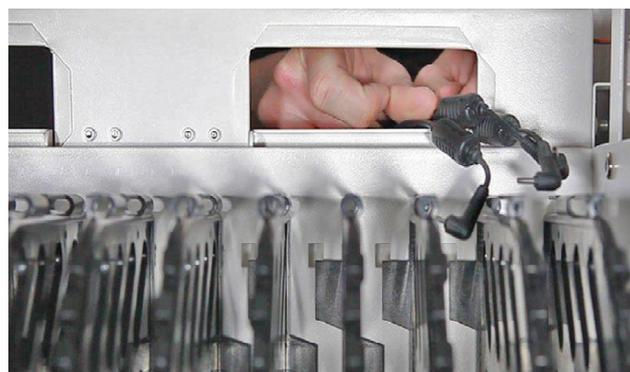
**Step-3:** Hook basket(s) in place & distribute power cords so that all power strips have an equal number of devices plugged in.
