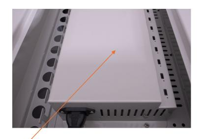
Charging hub with 65watts of power per port.
