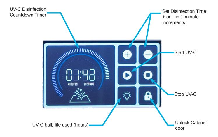
UV-C bulb life is monitored by the bulb life countdown meter. Press the "bulb" icon to see the number of hours bulb has been in use.
