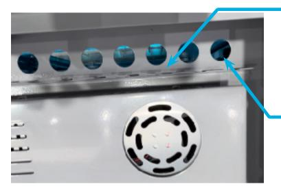
Wrap excess cable around strain relief bar tabs to adjust cable length.
