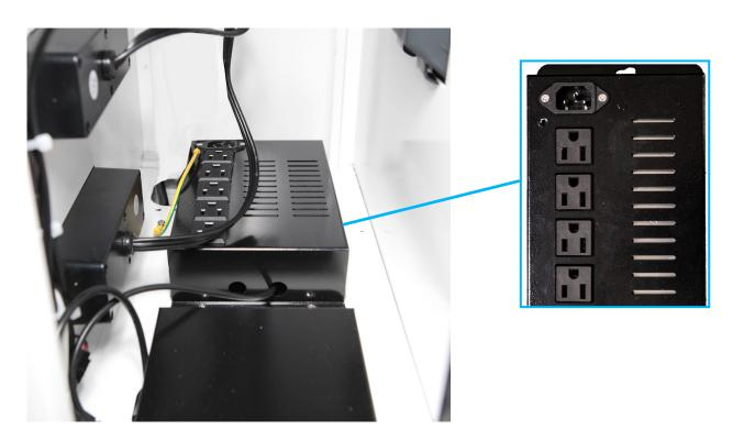
**Step-7:** One at a time, feed the Power Input Plug, then the Power Strip Plug through the pass-through hole located near the back.
